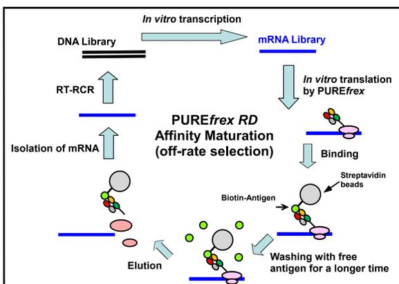
In off-rate selection, RD complexes bound to antigen-immobilized streptavidin beads were washed with large excess of free antigen to prevent the rebinding of RD complexes to the beads. The higher-affinity binders can be retained on the beads for a longer washing time.
